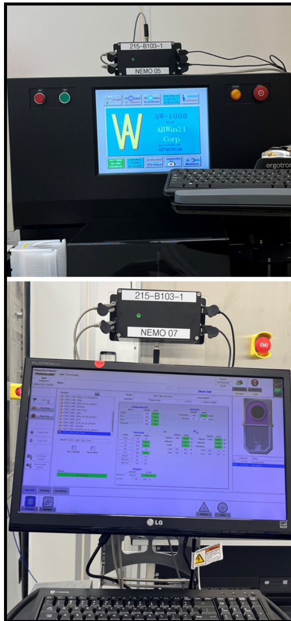
Figure 2.13: Examples of a dual-USB custom interlock control box mounted on top of an instrument and on top of a computer cart, as shown in the top and bottom images, respectively.
