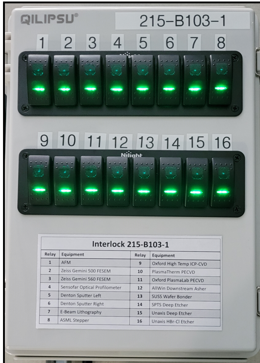
Figure 2.2: Front view of the interlock module showing the 2-way switches.
