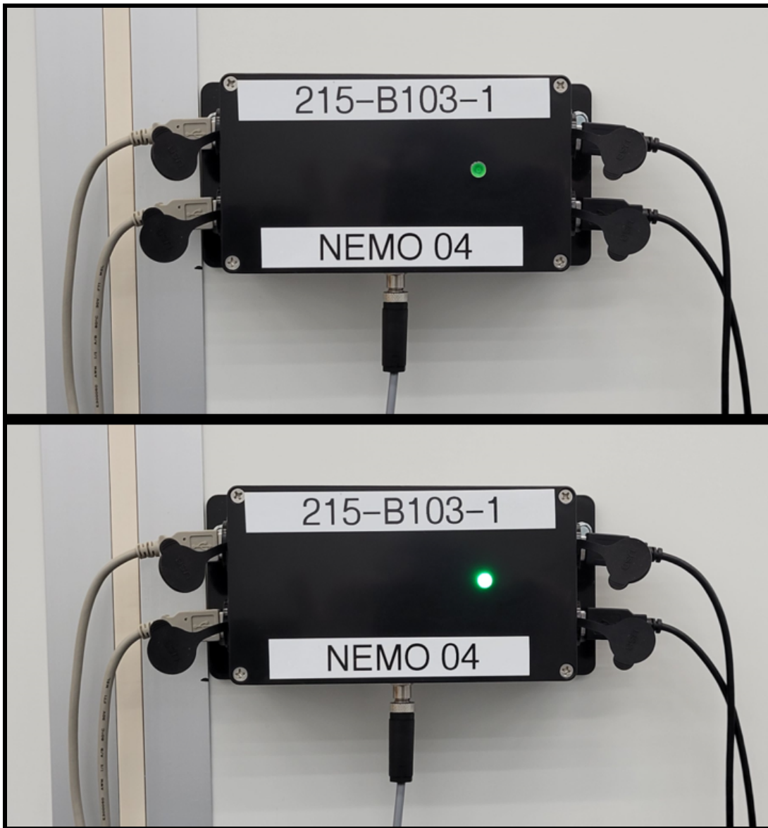
Figure 2.12: Example of a cleanroom wall-mounted dual-USB custom interlock control box in the disabled and the enabled state, as shown in the top and bottom images, respectively. The green LED lights up when the interlock is in the enabled state, as shown in the bottom image.
