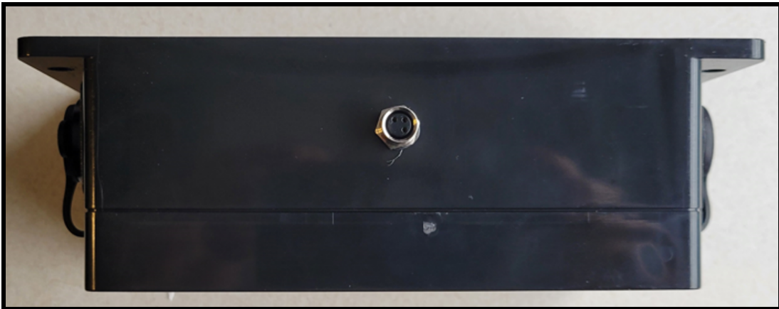
Figure 2.9: Top view of the dual-USB custom interlock control box showing the input control connection.
