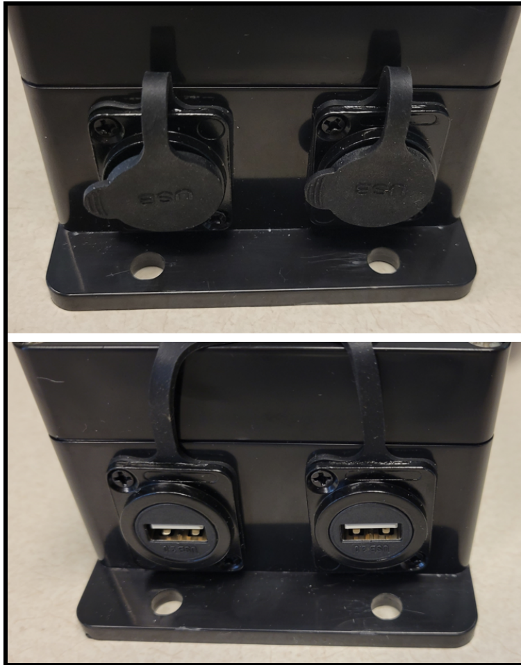
Figure 2.10: Side view of the dual-USB custom interlock control box showing the 2 USB connections with (top image) and without (bottom image) covers, and 2 wall-mounting holes.
