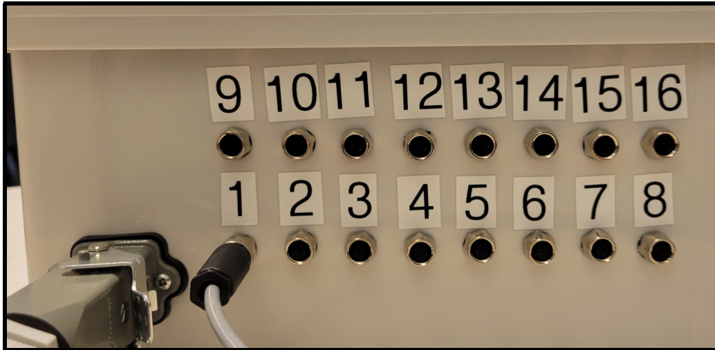
Figure 2.3: Bottom view of the interlock module showing the relay interlock outputs and the power cable connection.
