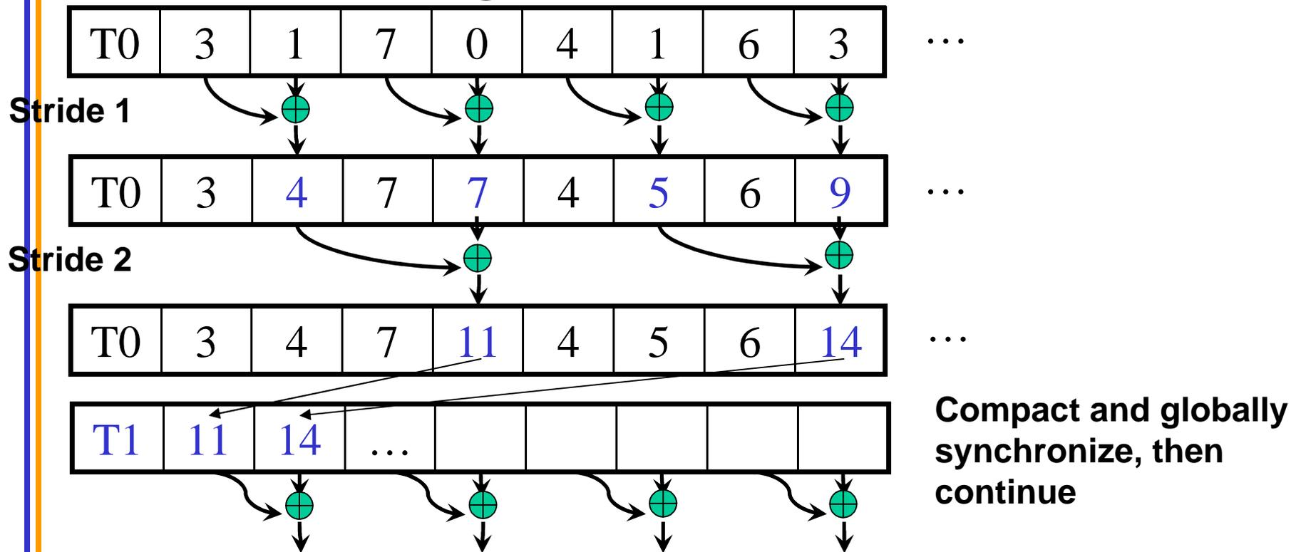
Iterate  $\log(n)$  times. Each thread adds value *stride* elements away to its own value.
