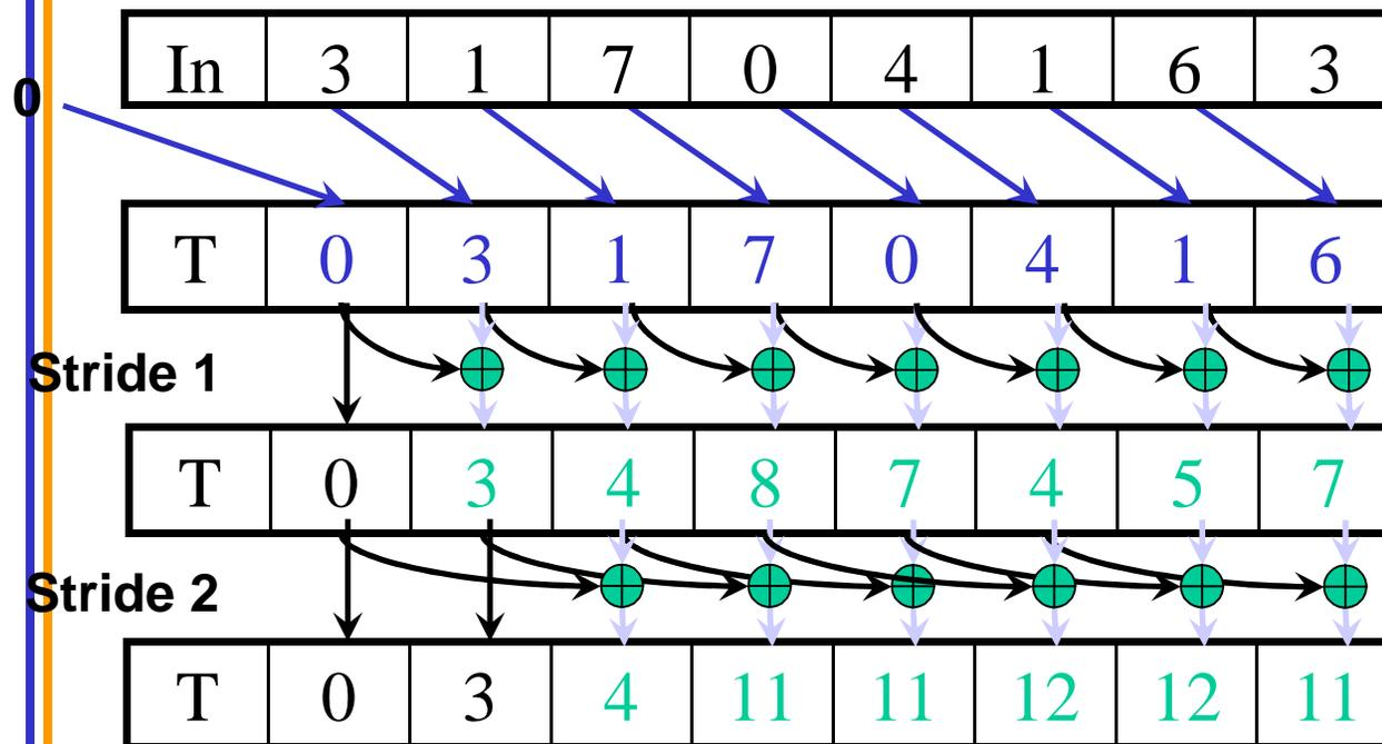
1. Read input from into a temporary array (shared memory in CUDA). Set first element to zero and shift others right.
