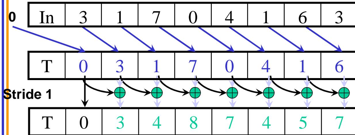
1. Read input from into a temporary array (shared memory in CUDA). Set first element to zero and shift others right.
