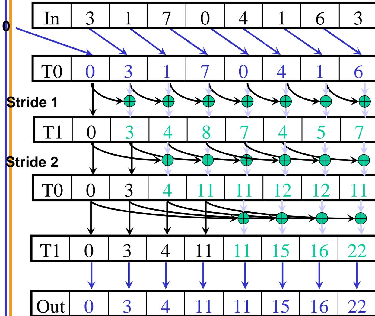
1. Read input from device memory to shared memory. Set first element to zero and shift others right by one.
