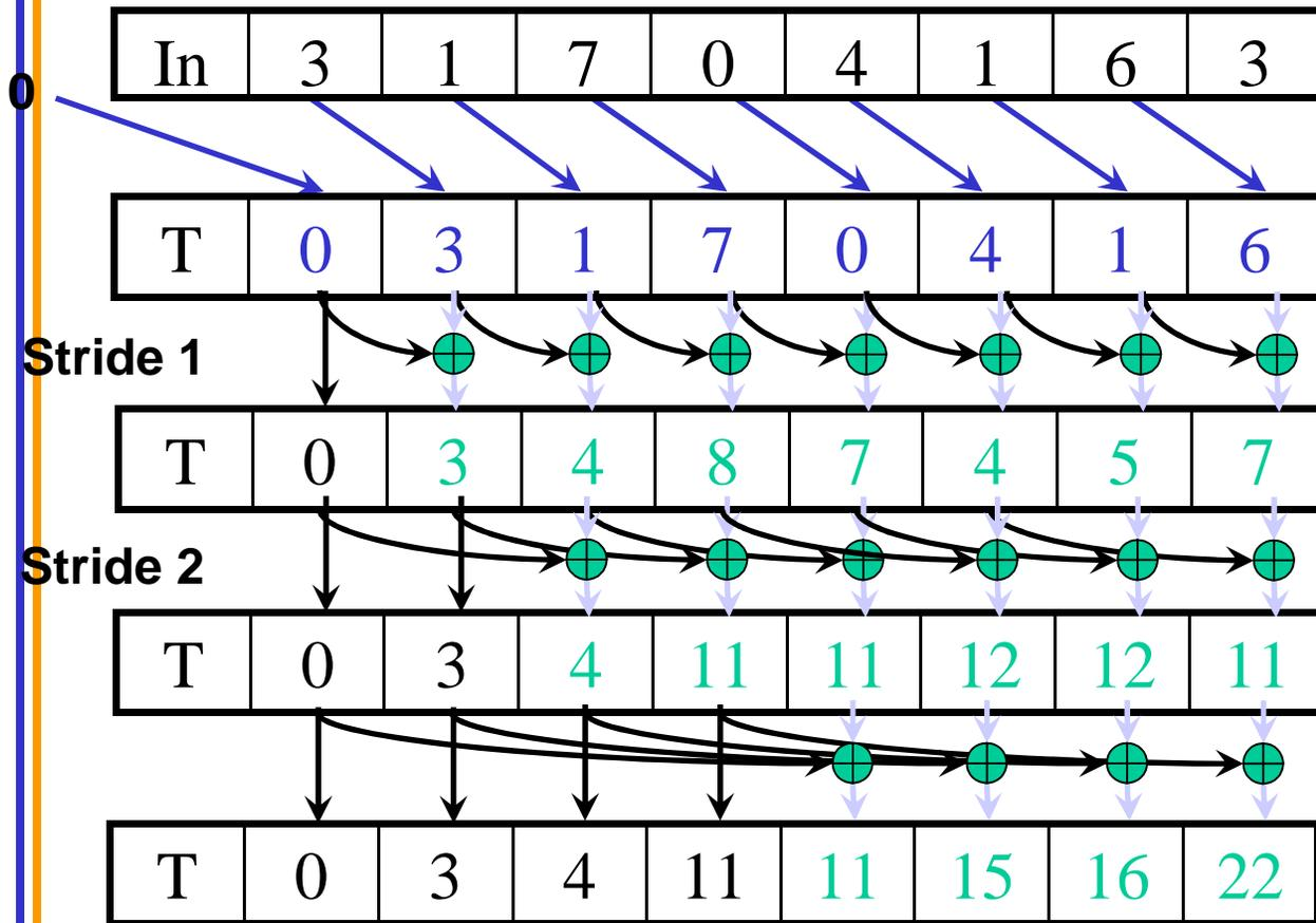
1. Read input from device memory to shared memory. Set first element to zero and shift others right by one.
