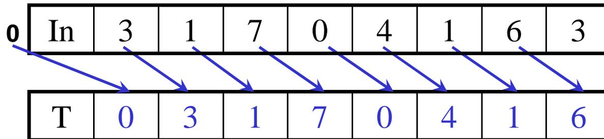
Each thread reads one value from the input array in device memory into shared memory array T0. Thread 0 writes 0 into shared memory array.
