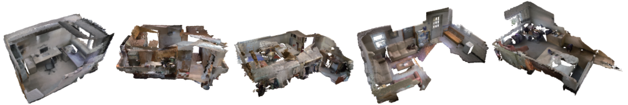
Figure 2: Mesh visualization. We use the generation and interpolation module to generate RGB images given depths/poses and then fuse them into mesh with TSDF fusion.
