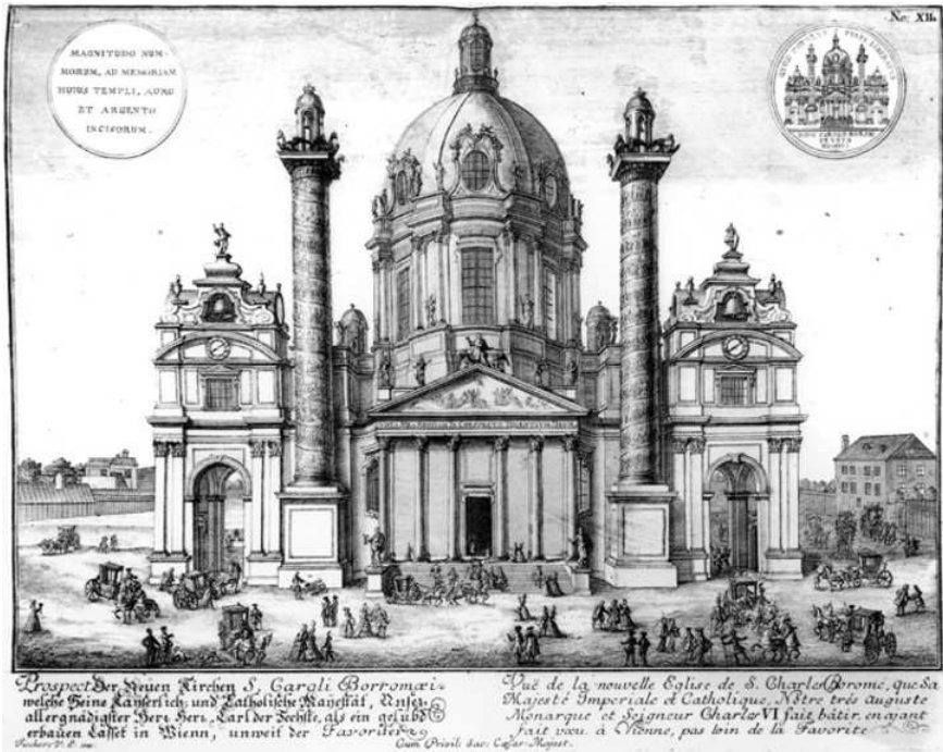
PLATE 30.7 Elevation of the Karlskirche, Vienna, by Fischer von Erlach. Plate 12 from his Entwurf of 1725. Note the twin spiral columns flanking the Antique Roman portico (Collection James Stevens Curl).
