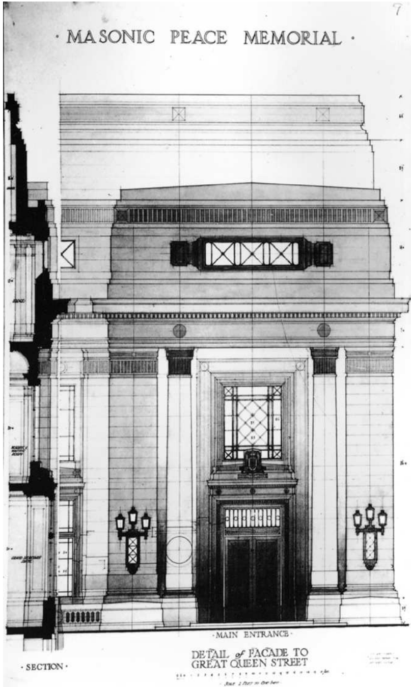
PLATE 30.21 Architects' drawing showing part of the treatment of the façade of the Masonic Peace Memorial, London (now known as Freemasons' Hall), with its in antis columns (United Grand Lodge of England).
