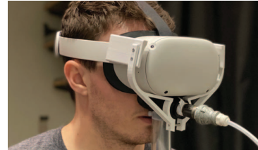
Figure 1: The Smell Engine enables programmable scent-filled environments, consisting of scenes and objects with associated odors that render through an olfactory display.
