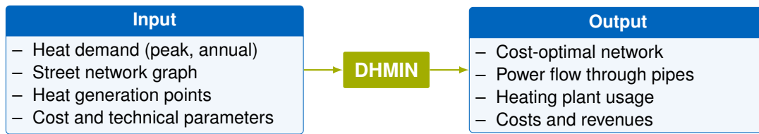
Figure 3.11: Input/output flow chart of model DHMIN
