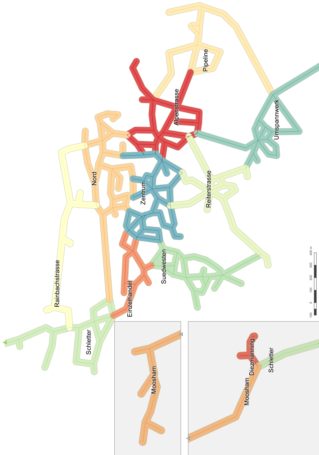
Figure 4.18: Map of 12 manually defined clusters for Haag i. OB. Vertices at edge borders form the boundaries between clusters.
