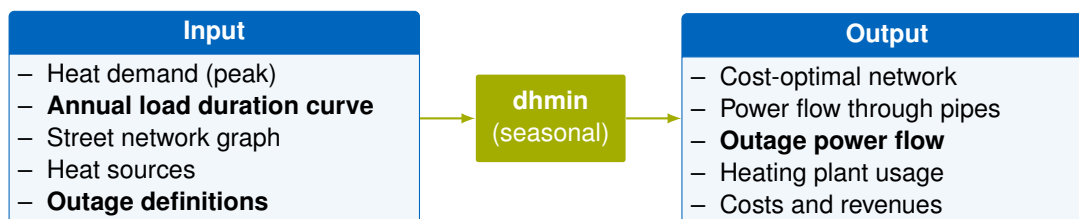
Figure 3.15: Input/output flow chart of model dhmin (seasonal). Differences to DHMIN in bold.
