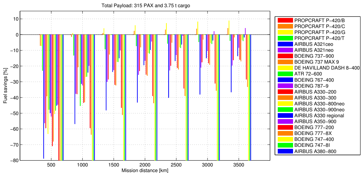
Figure 5.8.: Fuel savings [%] compared to the P-420/B for all mission distances and aircraft with a payload of 315 PAX and 3.75 t cargo
