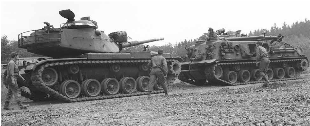
M60 tank being towed by an M88 armored recovery vehicle during REFORGER 78. (National Archives and Records Administration)
