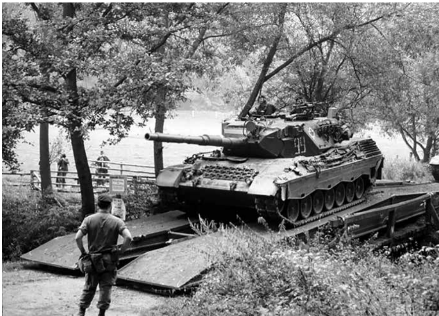
Canadian Leopard 1 crossing an obstacle courtesy of an armored bridgelayer. (Canadian Forces Combat Camera)
