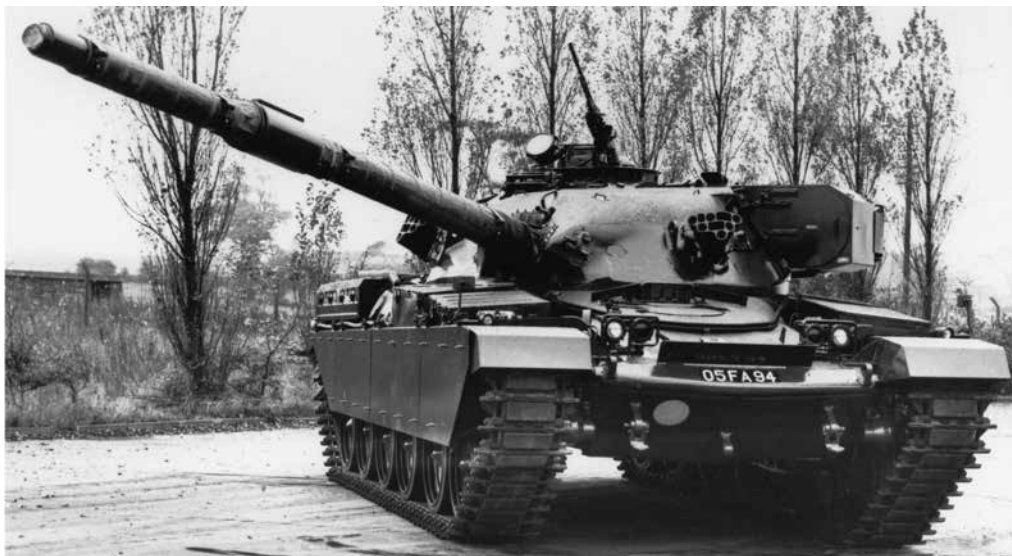
The lethal Chieftain with its 120-mm gun and heavy armor protection for its day. (U.S. Army Armor School Archives)
