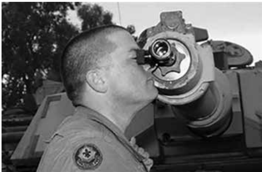
Using the in-bore muzzle boresight device. (Carl R. Johnson)
