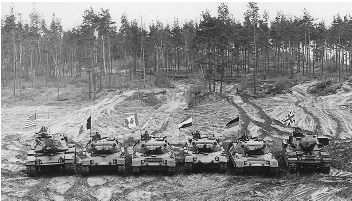
The competing steeds of CAT 77. From left to right they are an American M60A1, a Belgian Leopard 1, a Canadian Leopard 1, a Dutch Leopard 1, a German Leopard 1, and Britain's Chieftain. (Ron Mihalko)
