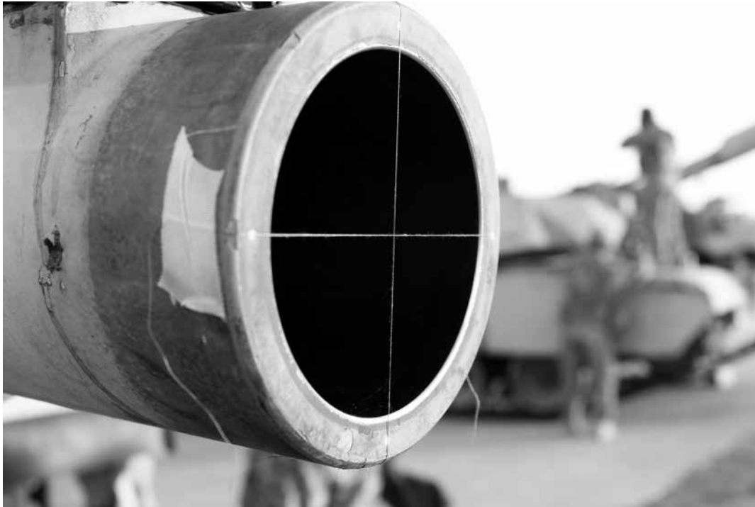
Old fashioned boresighting with tape and thread. (U.S. Army Armor School Archives)
