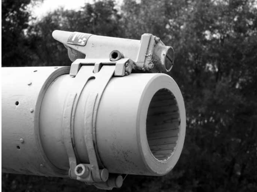
Close-up shot of part of the Muzzle Reference System, in this case the muzzle reference sensor that helped the gunner to determine and adjust for gun tube bend and droop. (Author)
