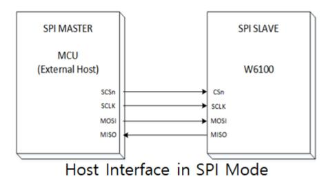
In serial bus mode, You should transmit and receive synchronously to SCLK the SPI signals such as MOSI and MISO from MSB to LSB of Register Offset Address bits, Block Select bits (**BSB**), R/W bit (**RWB**), **OP** Code bits and Read/Write 8bit Data.
