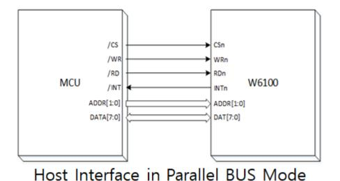
In parallel bus mode, You can access W6100 indirectly with **IDM\_AR0** (Indirect Mode Address Register 0), **IDM\_AR1** (Indirect Mode Address Register 0), **IDM\_BSR** (Indirect Mode Block Select Register), and **IDM\_DR** (Indirect Mode Data Register) specified with **ADDR0 & ADDR1**.
