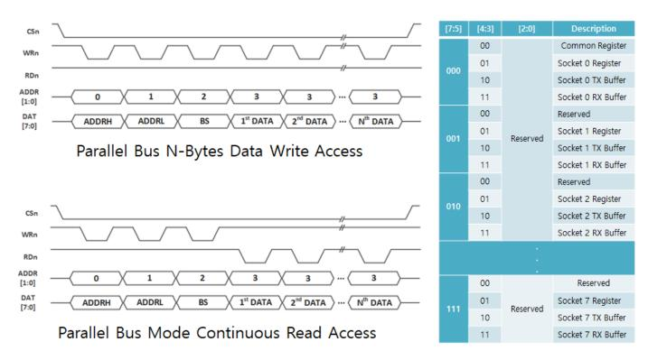
As following table shown, IDM\_BSR is used to select COMMON register block, 8 SOCKET register blocks and 8 SOCKET TX/RX buffer blocks.
