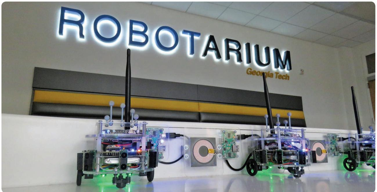
**FIGURE 2** A group of GRITSBot X robots charging on the inductive charging stations surrounding the Robotarium.
