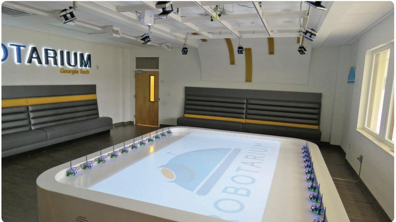
**FIGURE 1** The Robotarium testbed with GRITSBot X robots charging around the perimeter.
