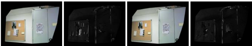
Fig. 7. (a) Model built from features selected by the user. (b) Birchfield dissimilarity per pixel from this model. White areas have a high dissimilarity value. (c) Refined model. (d) Birchfield dissimilarity after automatic model refinement
