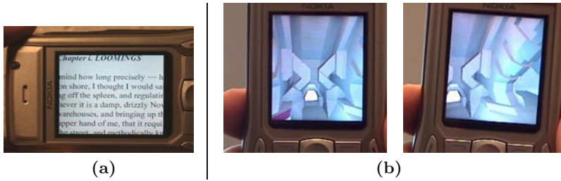
Fig. 4. (a) Camera-based interaction in a document viewing application. (b) Mapping physical motion to viewing direction creates the illusion of a window into an environment
