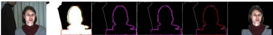
Fig. 5. (a) Input image (b) Segmentation result shown in white. Foreground contour from previous frame visualized on top. (c-d) Initial contour is moved towards new position. (e) Contour is fit to the contour of the segmentation. (f) Final foreground segmentation
