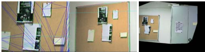
Fig. 2. Left: The Delaunay triangulation for the currently selected point pairs. Quickly zooming in allows for faster and more accurate operation. Middle: Corners and edges visualized on the reference backgrounds. Right: Partially completed rough 3D model, seen from an extrapolated viewpoint at the left side of the inputs
