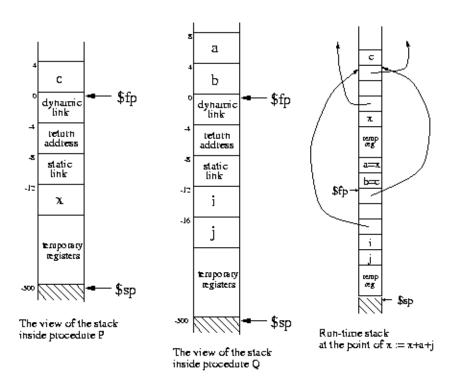
The activation record for Q (as Q sees it) is shown in the second figure above. The third figure shows the structure of the run-time stack at the point where x := x+a+j is executed. This statement uses x, which is defined in P. We can't assume that Q called P, so we should not use the dynamic link to retrieve x; instead, we need to use the static link, which points to the most recent activation record of P. Thus, the value of variable x is computed by:
