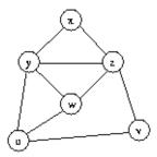
The nodes are pushed in the stack in the order of xvuzyw. Then, at the selection phase, xyzwuv variables are assigned the registers  $R_0R_2R_1R_0R_1R_0$ .
