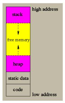
All dynamically allocated data are stored in the heap. These are the data created by malloc in C or new in C++. You can imagine the heap as a vector of bytes (characters) and end\_of\_heap a pointer to the first available byte in the heap:
