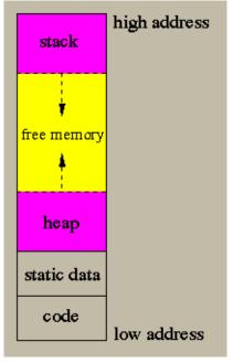
This is the layout in memory of an executable program. Note that in a virtual memory architecture (which is the case for any modern operating system), some parts of the memory layout may in fact be located on disk blocks and they are retrieved in memory by demand (lazily).
