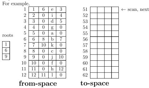
After we forward the roots from the from-space to the to-space, the to-space will contain the forwarded roots, and the roots and the forward pointers of the root elements in the from-space will point to the to-space, as shown below:
