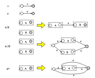
As it can been shown inductively, the above rules construct NFAs with only one final state. For example, the third rule indicates that, to construct the NFA for the RE AB, we construct the NFAs for A and B, which are represented as two boxes with one start state and one final
