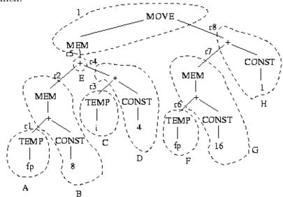
The order of tiling is IEHBDGACF (ie, top-down). After we set the tiles, we use a different register ri for each connection between the tiles. Then we expand the tiles into MIPS code by following the tile mapping table. The order of tile expansion is ABCDEFGHI (ie, bottom-up). The MIPS code is:
