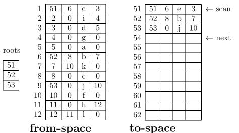
Then, we forward the pointers of the first element of the to-space pointed by the scan pointer (element 51). The first pointer 6 has already been forwarded to 52, as we can see from the element 6 in the from-space. The second pointer 3 is forwarded at the end of the to-space
