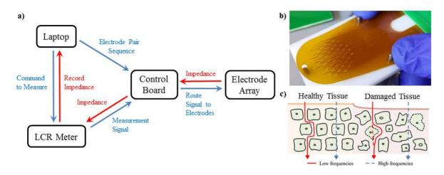
Figure 1. a) Overview of the impedance measurement system. b) 0.7-inch flexible electrode array board with hydrogel applied selectively to each electrode. c) Schematic of how low and high frequency signal travels through healthy and damaged tissue.
