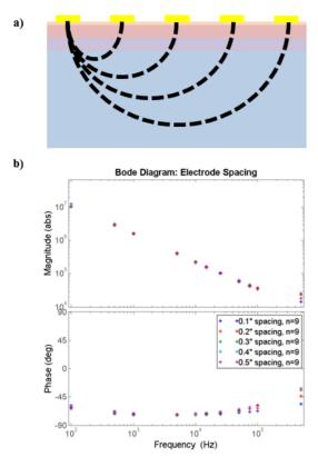
**Figure 2.** a) Schematic of penetration depth as a function of electrode spacing. b) Impedance magnitude and phase do not change significantly with respect to electrode spacing.
