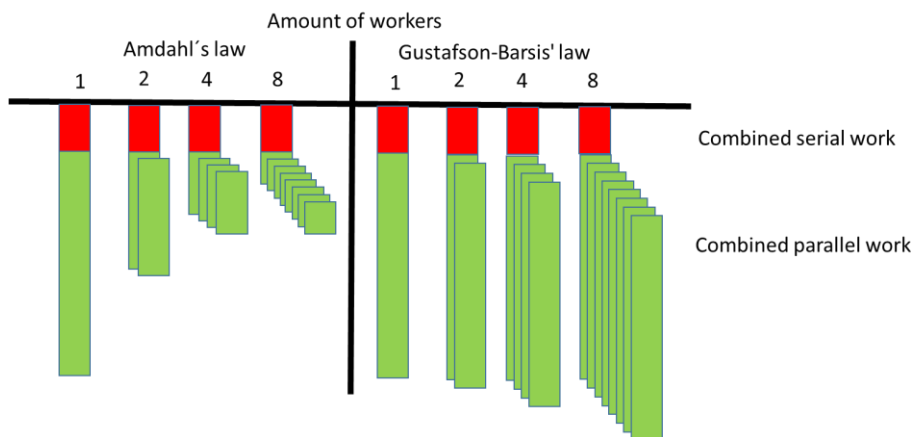
Figure 4 Amdahl and Gustafsson-Barsis' law view on combined work (McCool, Robinson, & Reindeer, 2012, pp. 59,62)
