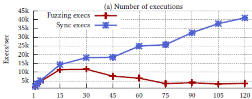
Figure 9 Multicore scalability of AFL according to Xu et al. (Xu, Kashyap, Min, & Kim, 2017, p. 4)
