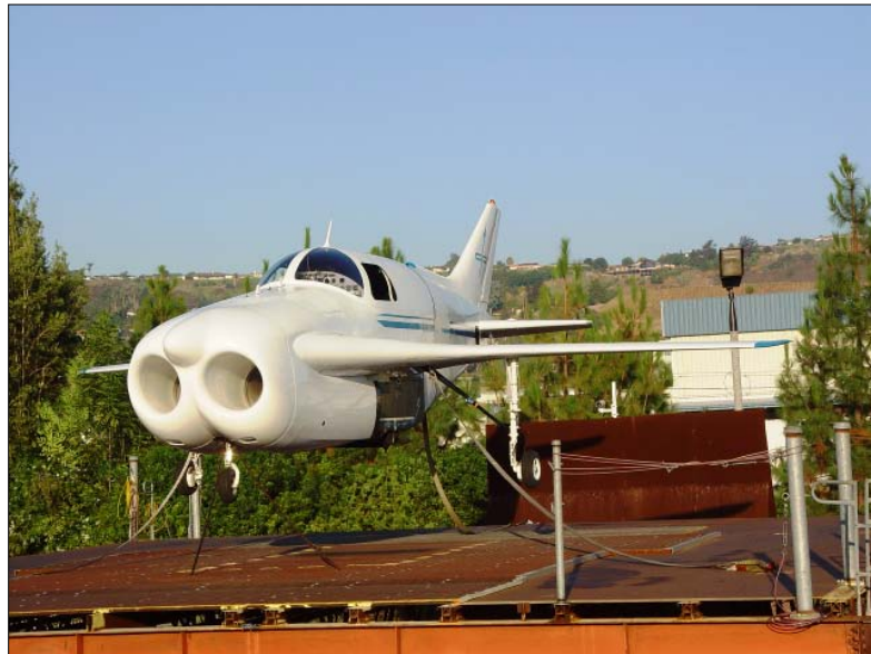
Figure 2. duPont Aerospace DP-1 in a tethered hover test. (Courtesy of duPont Aerospace Company)
