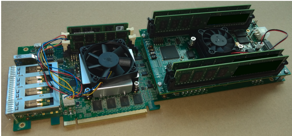
FIGURE 2.2: DFC equipped with FPGA Board (2a) and NAND DIMMs
