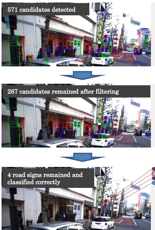
Fig.5 Results of detection, filtering and classification. In the images, box means region of road sign, and color of box means the color of road sign.
