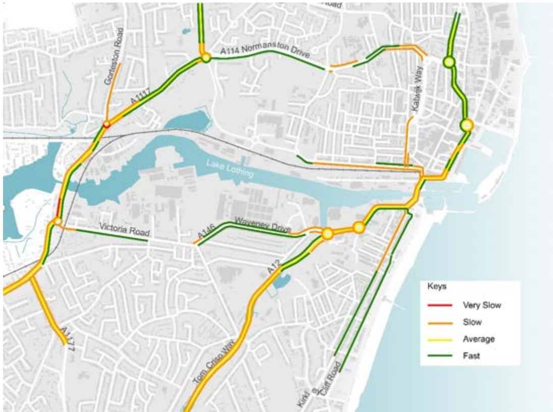
Figure 2-16: Typical Tuesday morning (8:30 a.m.) floating vehicle data on the approaches to the existing lake crossings (Source: Google Maps)
