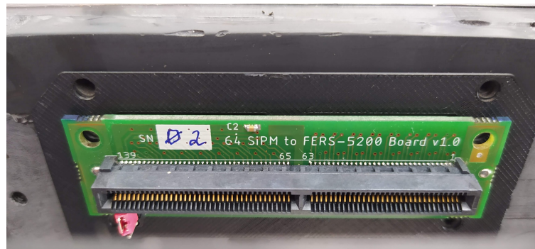
Front end board housing 64 SiPM
