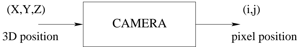
Fig. 5. From a geometric point of view, a camera converts a 3-D point (X, Y, Z) to a 2-D image point (i, j) .
