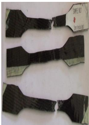
Fig.8 Fractured Tensile Specimens
