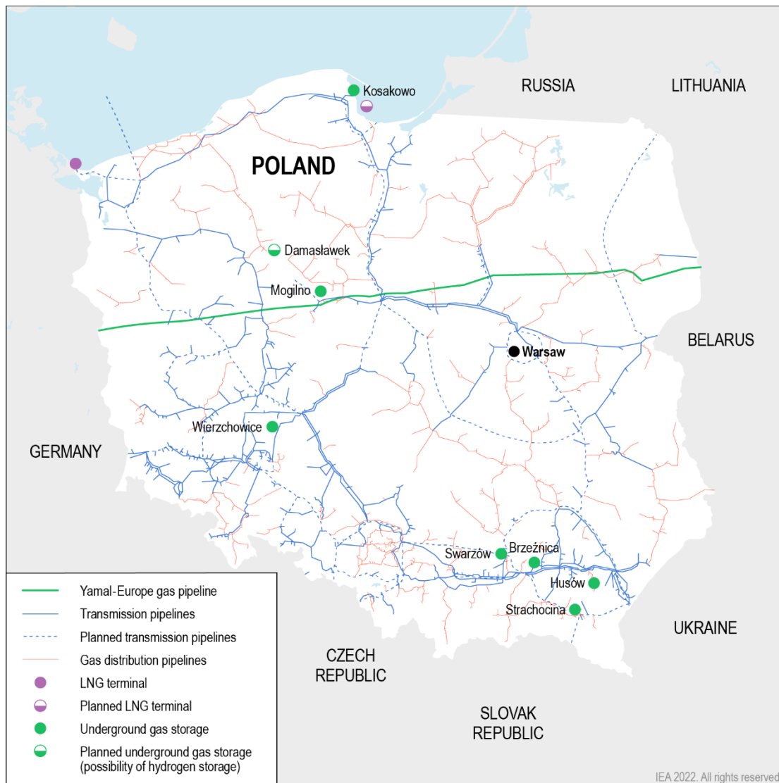
Figure 9.4 Poland's natural gas transmission system, 2020
