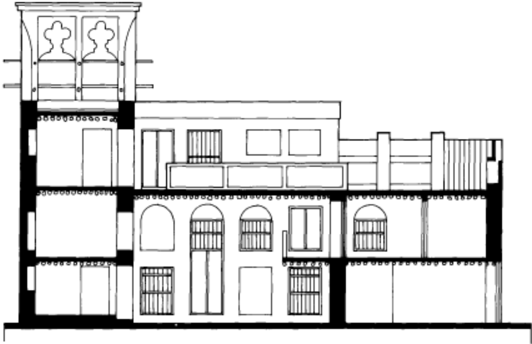
Traditional house, UAE. Note wind-tower (mulqaf) (after Kay and Zandi)
