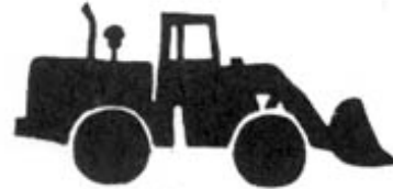
Articulated Loader (pivots in center)
