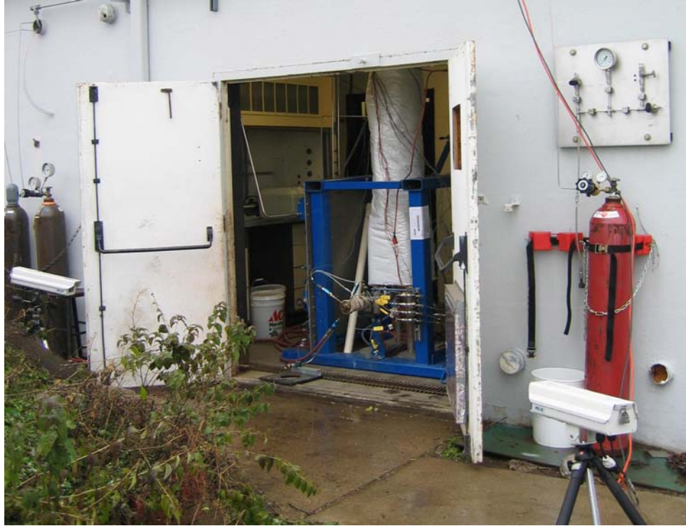
Figure 1 – View Looking Into Test Cell of Test Stand (Blue Frame and White Insulation Blanket Over Run Tank). Test Article (Gas Generator) is Mounted Horizontally (Approximately Picture Center).
