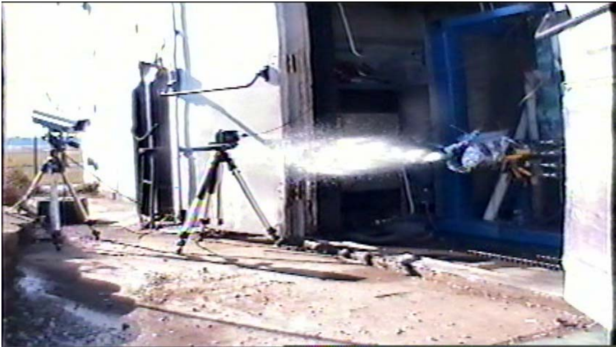
Figure 10 – Start Transient for PU010908_002 (0 °F H 2 O 2 , 35 °F GG Start Temp)
