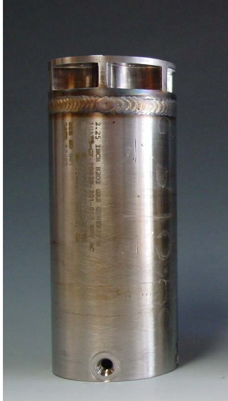
Figure 3 – 82-81% H 2 O 2 Gas Generator P/N: GK-PD039-201-003. GG is ~3 Inches (7.6 cm) in Diameter. Bottom is Exhaust End, One of the Four Instrumentation Ports are Shown In Photo.
