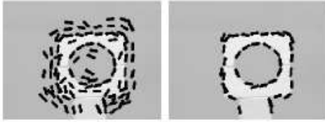
Figure 10: Different wavelets sharing the orientation of the feature in the image (left). Best ones automatically selected (right) (extracted from Krueger 2002 [5])
