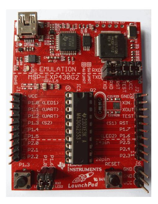
MSP-EXP430G2, LAUNCHPAD, DEV KIT Core Sub-Architecture: MSP430 Kit Contents: LaunchPad Emulator, Mini USB-B Cable, Quick Start Guide
