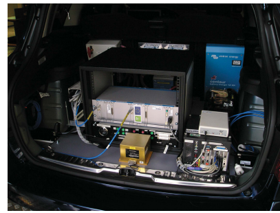
Figure 5. Embedded electronics and computer in the trunk
