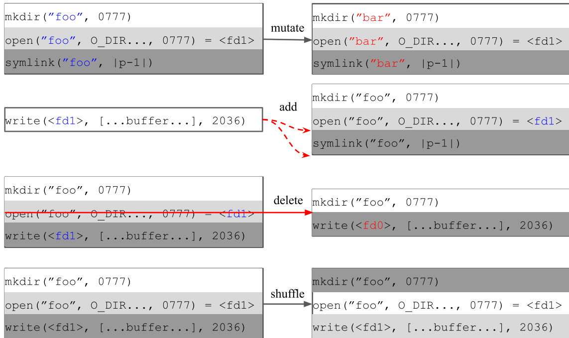
Figure 3.3: Illustration of four basic syscall sequence evolution strategies supported in KRACE: mutation, addition, deletion, and shuffling. For KRACE, each seed contains multi-threaded syscall sequences and each thread trace is highlighted in different shades of greyscale.
