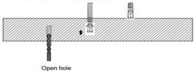
Fix the base of ropes onto wall or ceiling
