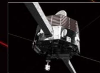
Mercury Magnetospheric Orbiter (MMO) developed by JAXA. The rod-shaped component visible is the magnetometer mast. (© JAXA)
