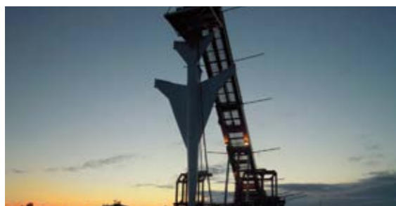
The D-SEND#2 experimental aircraft being lifted up by a mobile crane in preparation for the balloon launch. The aircraft was affixed to the balloon's gondola for the drop test. © JAXA
