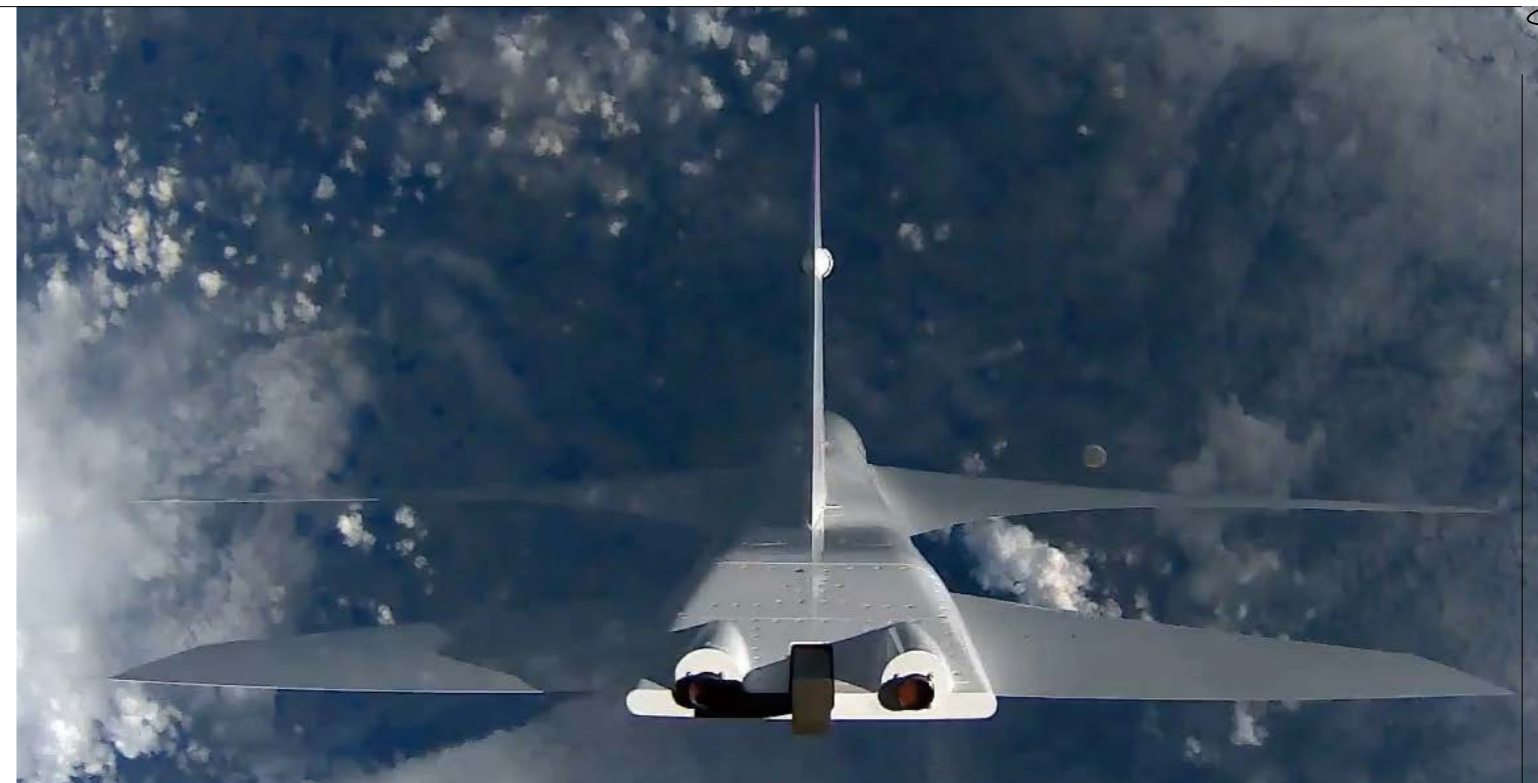
The moment at which the D-SEND#2 experimental aircraft—named the Silent SuperSonic Concept Model (SSCM)—was released from a balloon at an altitude of 30.5 km © JAXA
