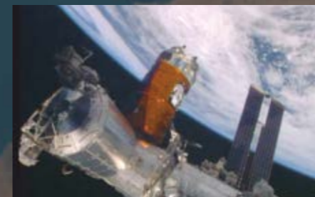
H-II Transfer Vehicle (“KOUNOTORI”) 5 (HTV5) HTV5 berthed to the Harmony Module (Node 2) of the ISS (© JAXA / NASA)
