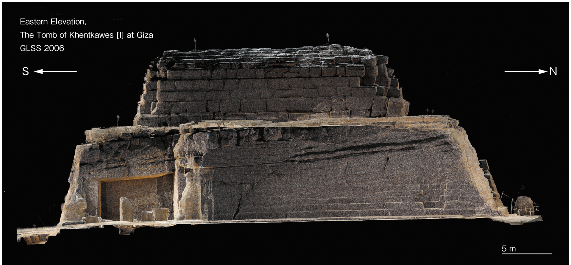
Fig. 4 Orthophotograph of the eastern elevation of the tomb, © Giza Laser Scanning Survey 2006.
