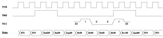
The IR code **1001** is shifted into the IR. After setting this IR code, it is now possible to write a 16-bit value to the specified bus address and bank:
