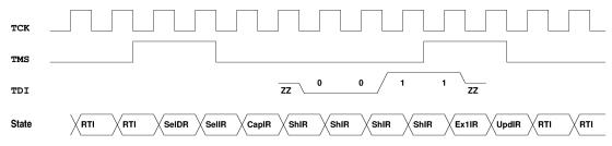
The JTAG TAP Controller state sequence starts in the *Run-Test/Idle* state. The IR code **1100** is shifted into the IR (least-significant bit first). After setting the IR code, it is now possible to set the bus address via a DR-Shift Sequence:
