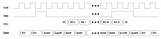
Here bits 15..0 define the 16-bit value to be written to the address specified by bits 31..16.
