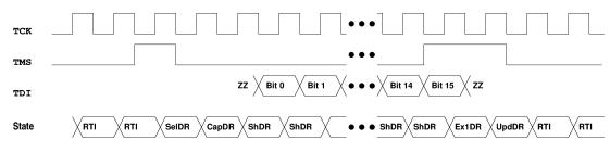
Bit 2..0 of the 16-bit value are used to set the address, bit 15..12 are used to set the bank. To execute a write access, you next have to set the IR to another value:
