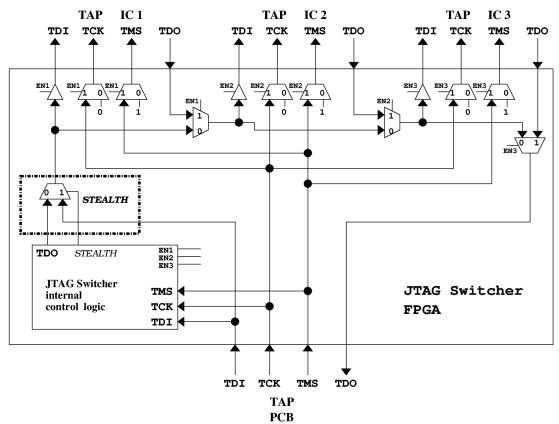
As depicted above: Once Stealth Mode is enabled, the TDI-TDO path of the JTAG Switcher TAP is bypassed. The effect is, that from the outside the JTAG Switcher TAP is not visible anymore.
