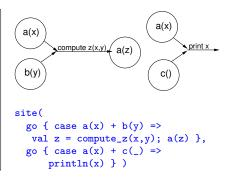
When a reaction starts: input molecules disappear, expression is computed, output molecules are emitted
