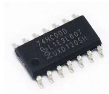
Figure 2.2.4: 74HC00 chip physical view
