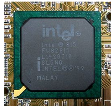
Figure 3.1.6: An Intel 82815 Graphics and Memory Controller Hub embedded on a PC motherboard. (Source: Wikimedia , author: Qurren)
