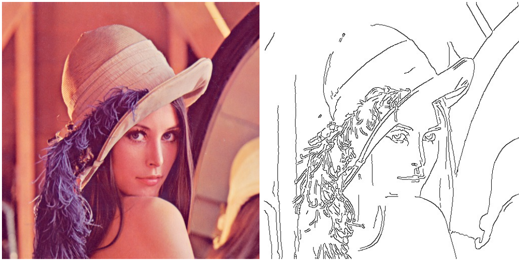
Figure 6.7: An example of the Canny algorithm applied to the Lena standard test image (left) which identifies edge pixels in the image (right).
