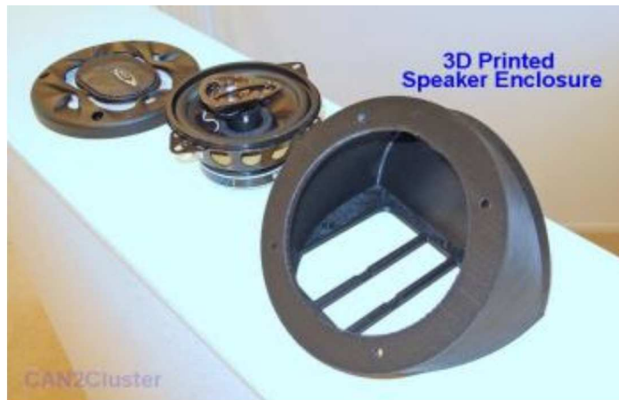
DiY 3D printed speaker
