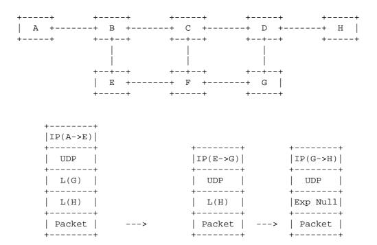
Figure 3: Packet Forwarding Example with PHP
