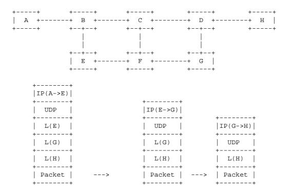
Figure 4: Packet Forwarding Example without PHP
