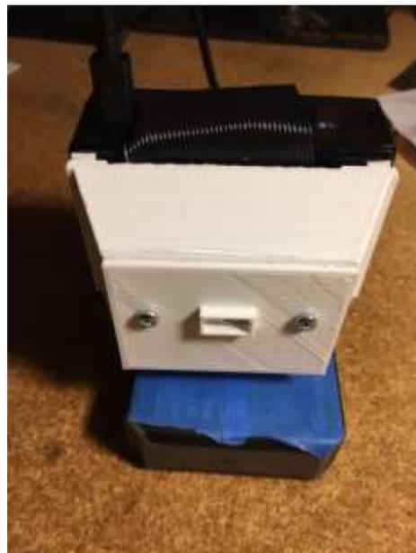
NOTE that you cannot cover the front lens of the AMG8833 as most glass or clear plastics will absorb the far-infrared, thus be opaque to the camera.
