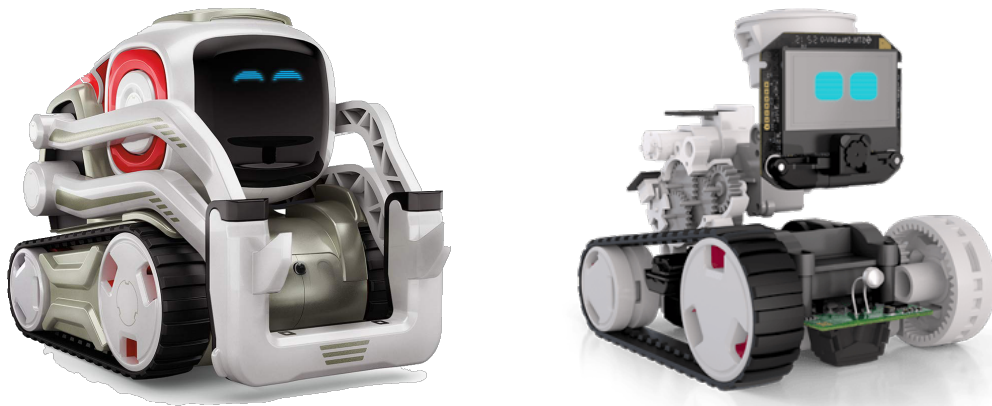
Figure 3.1. On the left there is a photo of Anki Cozmo in action, while on the right side there is a graphical reconstruction of the whole set of gears and hardware inside the robot.
