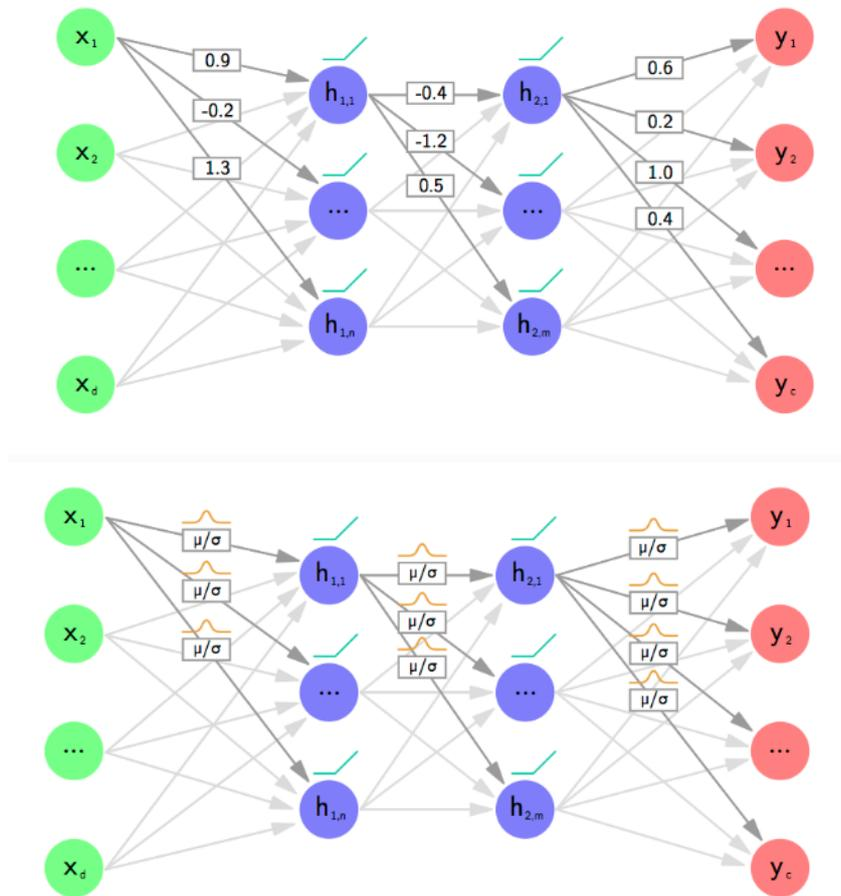
Fig. 1.1 Top: Each filter weight has a fixed value, as in the case of frequentist Convolutional Networks. Bottom: Each filter weight has a distribution, as in the case of Bayesian Convolutional Networks. [16]
