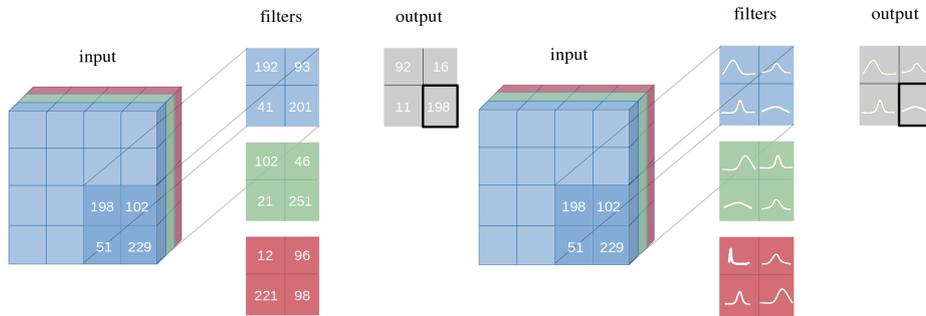
Fig. 4.1 Input image with exemplary pixel values, filters, and corresponding output with point-estimates (top) and probability distributions (bottom) over weights.[55]
