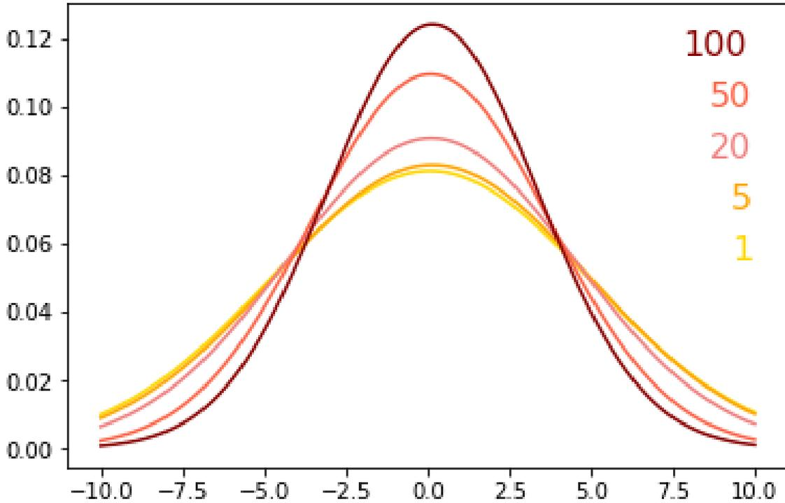
Fig. 5.3 Convergence of the Gaussian variational posterior probability distribution  $q_{\theta}(w|\mathcal{D})$  of a random model parameter at epochs 1, 5, 20, 50, and 100. CIFAR-10 is trained on Bayesian LeNet-5.
