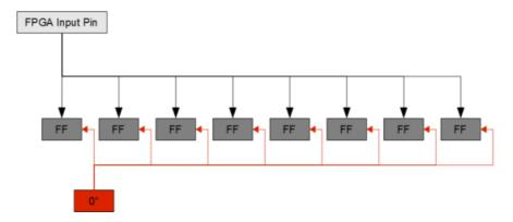
To reduce the length of the carry chain, it is driven by 400*MHz* instead of 200*MHz* and its 84 steps cover a bit more than 2.5*ns*. The 84 bits wide high resolution pattern received from the carry chain sampler is encoded into 7 bits, representing the position of the leading edge of the signal inside the chain, the desired high resolution time information. This implies, that only one leading edge within 2.5*ns* can be recorded (the first one).
