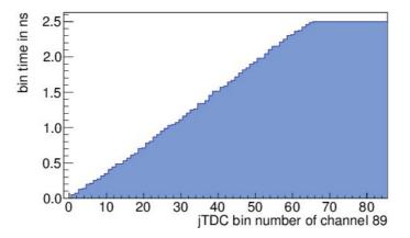
From this data one can obtain the time for each tdc bin. This offline calibration needs to be done for each tdc channel. For a detailed howto look at the source of *jAnalyzer*, which is doing just that.
