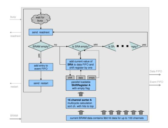
In order to get this done fast, the channels are pre-processed in groups of 16 and each group sorts the channels which contain hits to the top. The serializer queries each group and jumps to the next if done. By doing so, the serializer needs only 8 clk cycles to process a BRAM chunk containing just a single hit.
