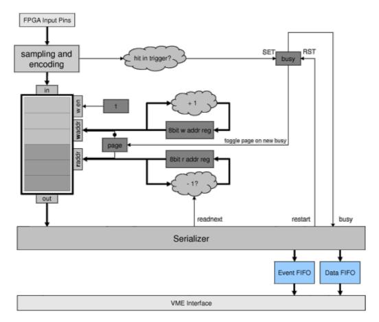
If the serializer is not able to push any more data in the FIFOs, because they are full (not beeing read out), it simply stops processing the BRAM, thus not issuing any readnext or restart commands. If the event is larger than the the DATA FIFO, the serializer has to truncate the event, because the EVENT
