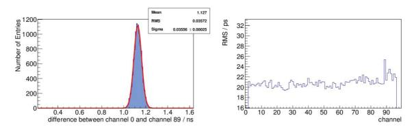
If the analog input card is used, time over threshold values from jTDC can be correlated to the pulse integral of an SADC (left plot). A standard ADC spectrum (without pedestal) can be extracted from the jTDC ToT data. Energy calibration is still needed (right plot).
