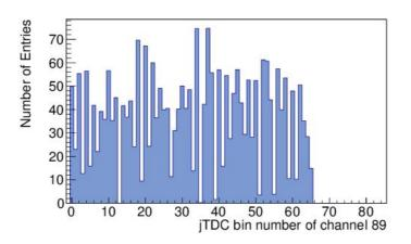
If we assume that the input data is white noise and that we have enough statistics, the above bin distribution can be used to calculate the individual width of each bin by normalizing the integral of the histogram to 2.5*ns*:
