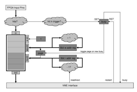
To prevent further page flipping until the read-from-page has been read-out completely, the page bit is locked until a "restart" command is send. So trigger inputs during read-out are ignored.
