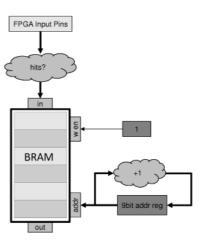
The read-out is controlled by sending "readnext" commands via VME, which decrements the 9bit-BRAMaddress. The currently addressed memory cell can be read via VME. After all data has been read by rewinding the BRAM, a "restart" command is issued which clears the busy flag and switches the BRAM back to recording mode.
