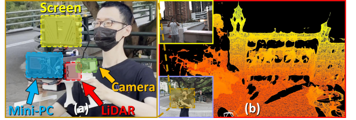
Fig. 6: (a) shows our handheld device for data collection and online mesh reconstruction. (b) shows a snapshot of our accompanying video [70] (starting at 00:09) of Experiment-1, with three time-aligned views of different sources including a screen-recorded view (in red), a camera preview (in yellow), and a third-person view (in blue).
