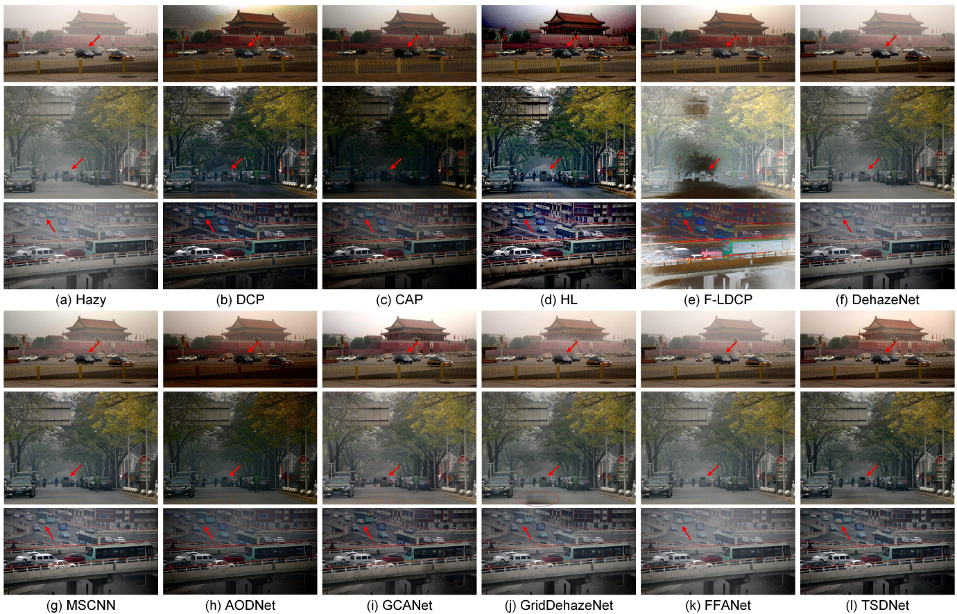
Fig. 4. Visual comparisons of various methods on three RESIDE-RTTS real-world images from Test-R. The proposed method can remove haze more fully on the premise of ensuring the natural scene.
