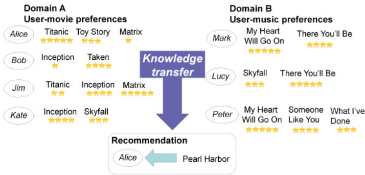
Fig. 12. An example of CDCF scenario. In Domain A, Alice’s preferences are not similar to any of the other users in this domain. However, in Domain B, we discover that users who like “My Heart Will Go On” (the theme song to Titanic ) may also like “There You’ll Be” (the theme song to Pearl Harbor ). This knowledge can be exploited for recommending the movie Pearl Harbor to Alice.
