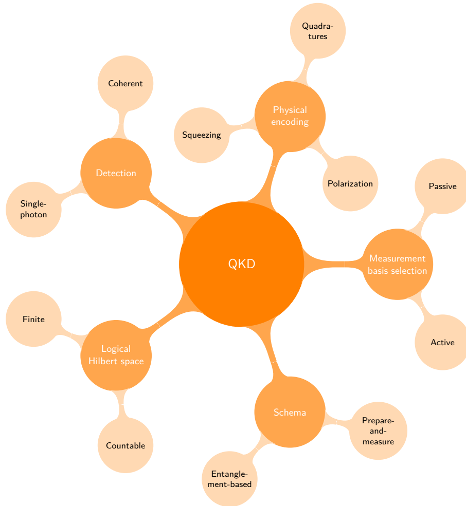
Figure 1.5.: Common characteristics of QKD protocols in a tree diagram. The protocol schema is either prepare-and-measure (P&M) or entanglement-based (EB). The Measurement basis selection is either passive or active. The detection is usually coherent or based on single-photon clicks. The logical Hilbert space is either finite or countable. Among many, the physical encoding uses the field quadratures, polarization, or squeezing degrees of freedoms (DOFs) of light.
