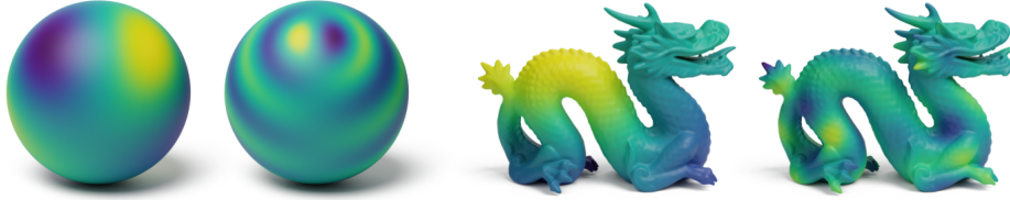
Figure 3.3. Eigenfunctions of the Laplace–Beltrami operator on a sphere and dragon manifold.
