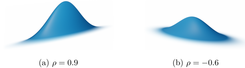
Figure 1.7. Two multivariate Gaussian densities, in dimension two, with unit variances and different correlation coefficients \rho . As |\rho| \rightarrow 1 , the individual components of the multivariate Gaussian become more and more dependent.
