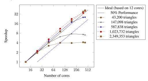
**Figure 16.3:** Speedups for problems ranging from 43,200 triangles to 2,349,353 triangles showing excellent speedups for the larger problems. We surmise that the super-scalability stems from better cache utilization as the larger meshes are subdivided into smaller meshes that can fit into cache.
