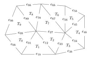
Figure 16.1: Triangular mesh used in our finite volume method. Conserved quantities h, uh and vh are associated with the centroid of each triangular cell,  $T_i$ . From the values of the conserved quantities at the centroid of a cell and its neighbouring cells, a discontinuous piecewise linear reconstruction of the conserved quantities is obtained. Fluxes are calculated across each edge  $e_{ij}$  using the reconstructed quantities.
