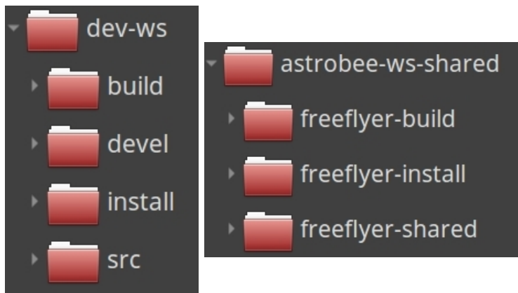
Figure 13: A standard Catkin workspace directory (left); the typical workspace setup used by the Astrobe Flight Software (right).
