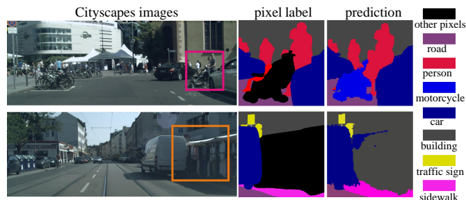
Fig. 1: We motivate open-set recognition with safety concerns in autonomous vehicles (AVs). Contemporary benchmarks such as Cityscapes [1] focus on K classes of interest for evaluation, ignoring a sizeable set of “other” pixels that include vulnerable objects like wheelchairs and strollers (upper row). As a result, most state-of-the-art segmentation models [2] also ignore these pixels during training, resulting in a stroller misclassified as a “motorcycle” (top) and a street-market misclassified as a “building”. Such misclassifications may be critical for AVs because these objects may require different plans for obstacle avoidance (e.g., “yield” or “slow-down”). Fig. 6 shows our approach, which explicitly augments state-of-the-art segmentation models with open-set reasoning.
